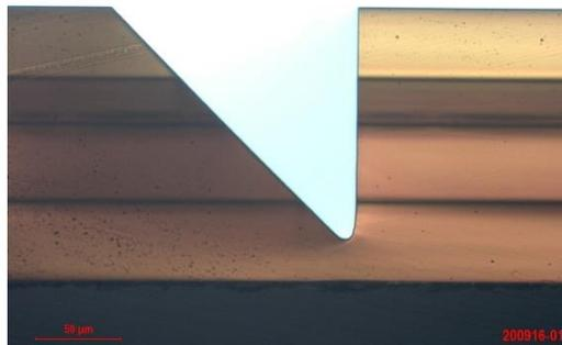
Figure 6. Side-view of the diced 45° mirrors for the coupling of the backside illuminated PDs required to implement the on-chip wavelength meters.
