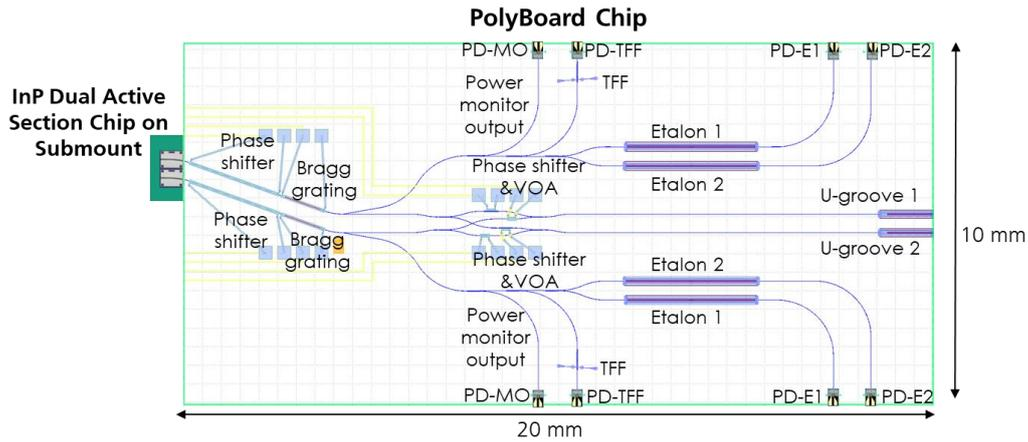
Figure 1. Schematic of the Photonic-based VNA signal source PIC based on Fraunhofer HHI's PolyBoard hybrid photonic integration technology. VOA: Variable optical attenuator; TFF: thin-film filter; PD-MO: photodiode for power monitoring; PD-TFF: photodiode in the thin-film-filter path; PD-E1: photodiode after the Etalon 1; PD-E2: photodiode after the Etalon 2
