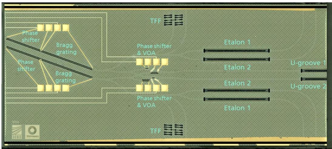
Figure 4. Picture of the fabricated PolyBoard chip for the photonic-based VNA signal source PIC. VOA: Variable optical attenuator; TFF: thin-film filter.
