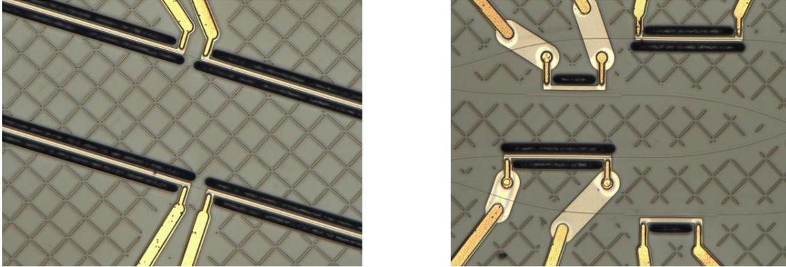
Figure 5. (Left) Picture of the phase shifter and Bragg grating sections of two tunable lasers. (Right) Detailed picture of the central PIC section that combines the two tunable lasers and comprises phase shifters and variable optical attenuators.
