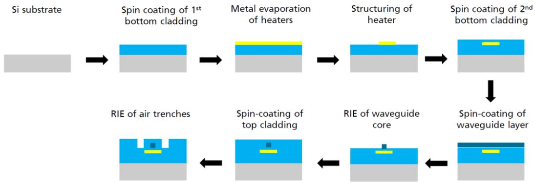
Figure 3. Schematic of Fraunhofer HHI's PolyBoard hybrid photonic integration chip structure [6].
