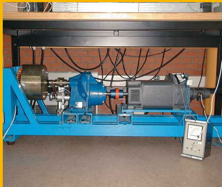
Motor – permanent magnets synchronous generator bank of the Power Control Group Research Laboratory.
