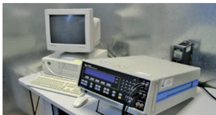
Equipment for characterising the dielectric response of insulating materials in the control of frequency. Band width/range 0,1 uHz at 30 MHz
