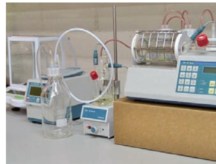
Karl-Fischer equipment for moisture-content titration in paper insulation for power Equipment for capacitance and tg measurements.
