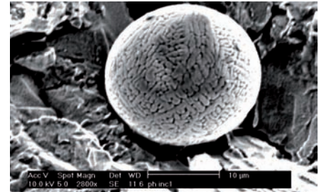
Stainless steel 17-4 PH particle treated by HIP (Hot Isostatic Pressing)
