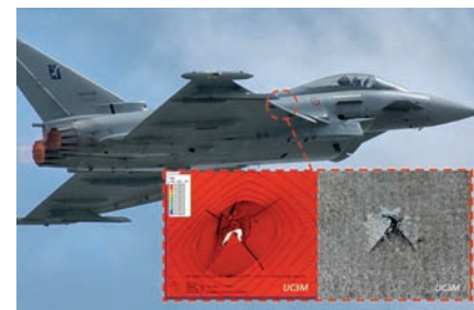
Simulation of a high-velocity impact on carbon fiber laminate.
