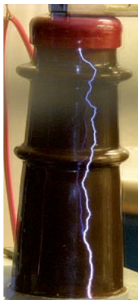
Applied voltage tests on an outdoor MV insulator
