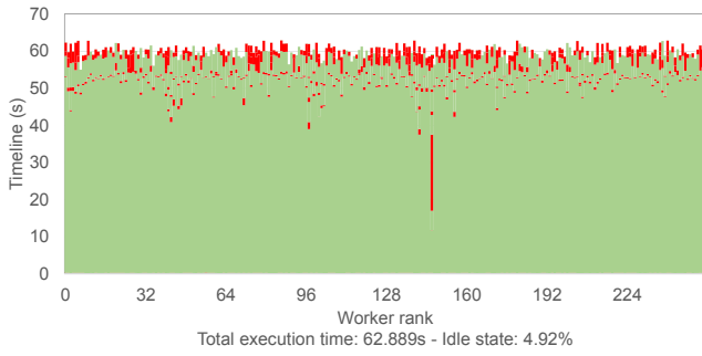
(a) Timeline in seconds for each worker, using default data-placement and locality-agnostic Swift/T scheduler.
