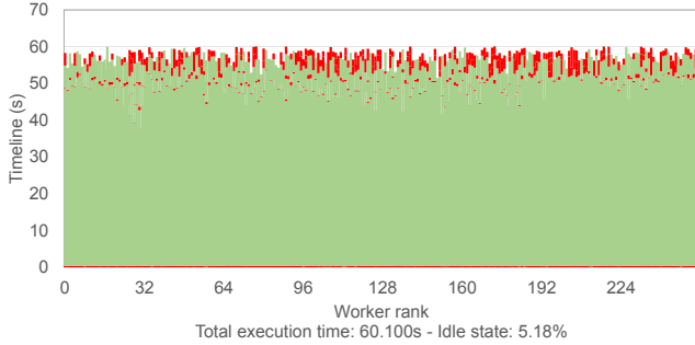
(c) Timeline in seconds for each worker, using default data-placement and best-effort locality-aware scheduling (SOFT, NODE).
